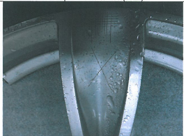
1#-2 Specimen after test(192h)
